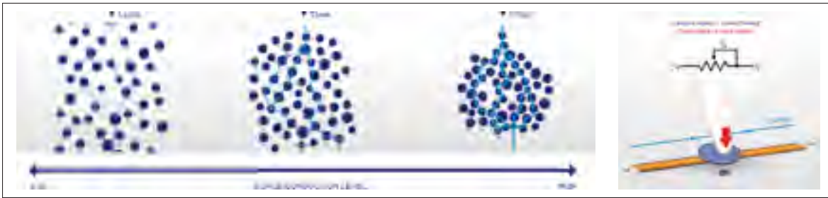
Figure 2.3 (a) Percolation effect in material under stress, (b) Model of the sensor based on QTC
