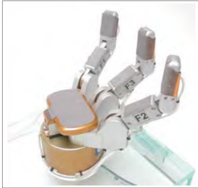
Figure 2.1 RoboTouch tactile sensors by PPS on Barette hand
