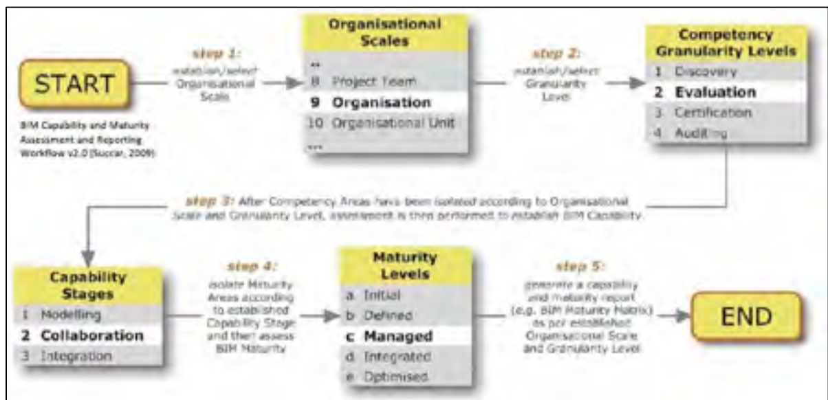
Figure 2.10 BIM capability and maturity assessment and reporting workflow diagram–v2.0 Taken from Succar (2010a) and Succar et al. (2012)
