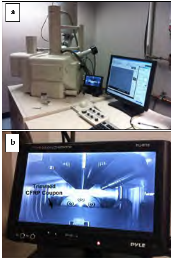
Figure 2.17 a) SEM - type Hitachi S-3600N, b) CFRP laminate in the vacuum chamber of scanning electron microscope
