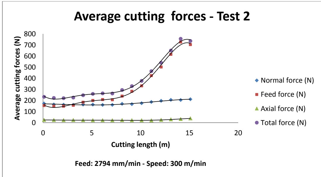
Figure 4.10 Average forces in x, y and z directions and average total forces as a function of cutting length in Test 2
