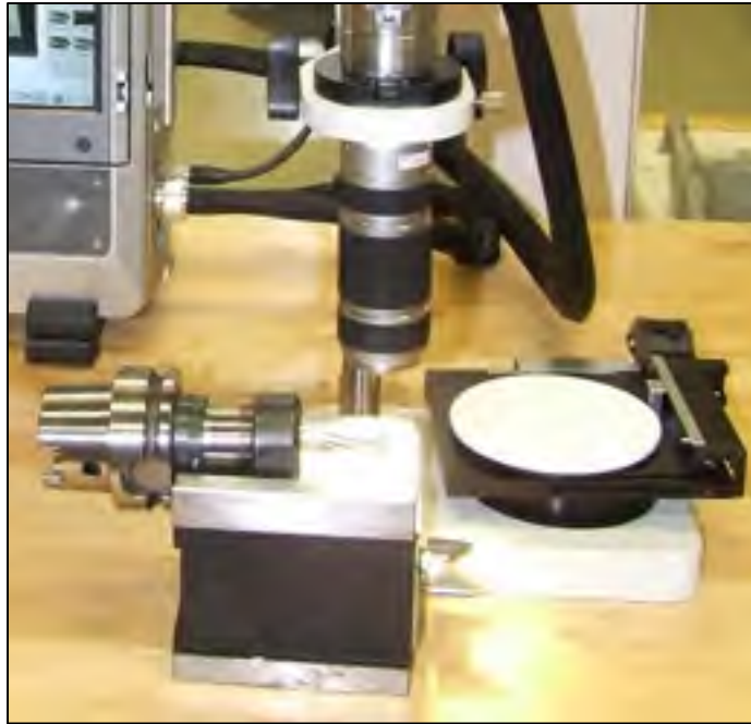
Figure 2.14 Tool holder including cutting tool mounted on magnetic clamp for tool wear measurement
