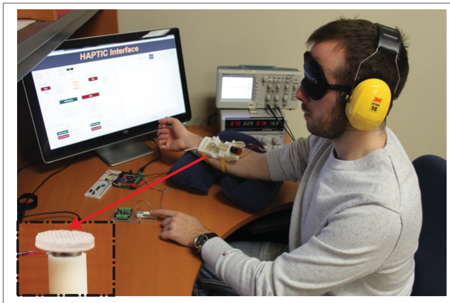
Figure 4.3 Participant applying pressure to the load-cell sensor while blindfolded and wearing the noise-removal headphones. The red arrow indicates a close-up view of the piston portion of the haptic device, with the circular unit attached to the top of the piston
