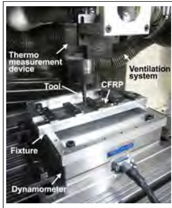
Figure 4-1 CFRP milling setup
