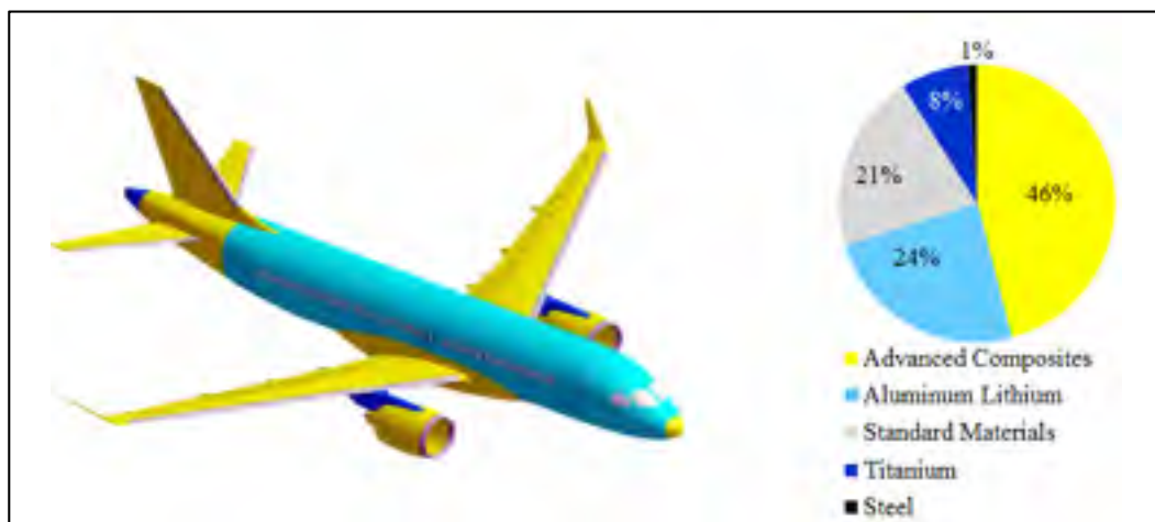
Figure 1-1 The application of composite materials in different parts of the Bombardier CSeries (Kafyeke, 2010)
