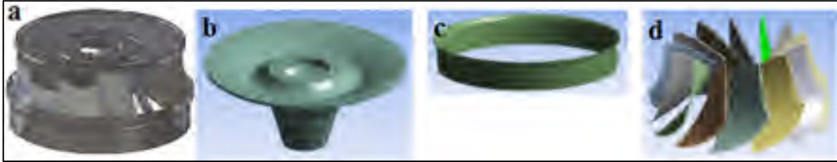
Figure 1-1 (a) Francis turbine runner (Boudreault et al., 2014) and components (b) crown, (c) band, and (d) blades, respectively from left to right (Saeed, Galybin et Popov, 2010)
