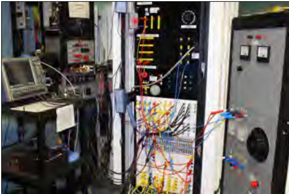
Figure 3.11 Transformerless-HSeAF prototype used for experiments
