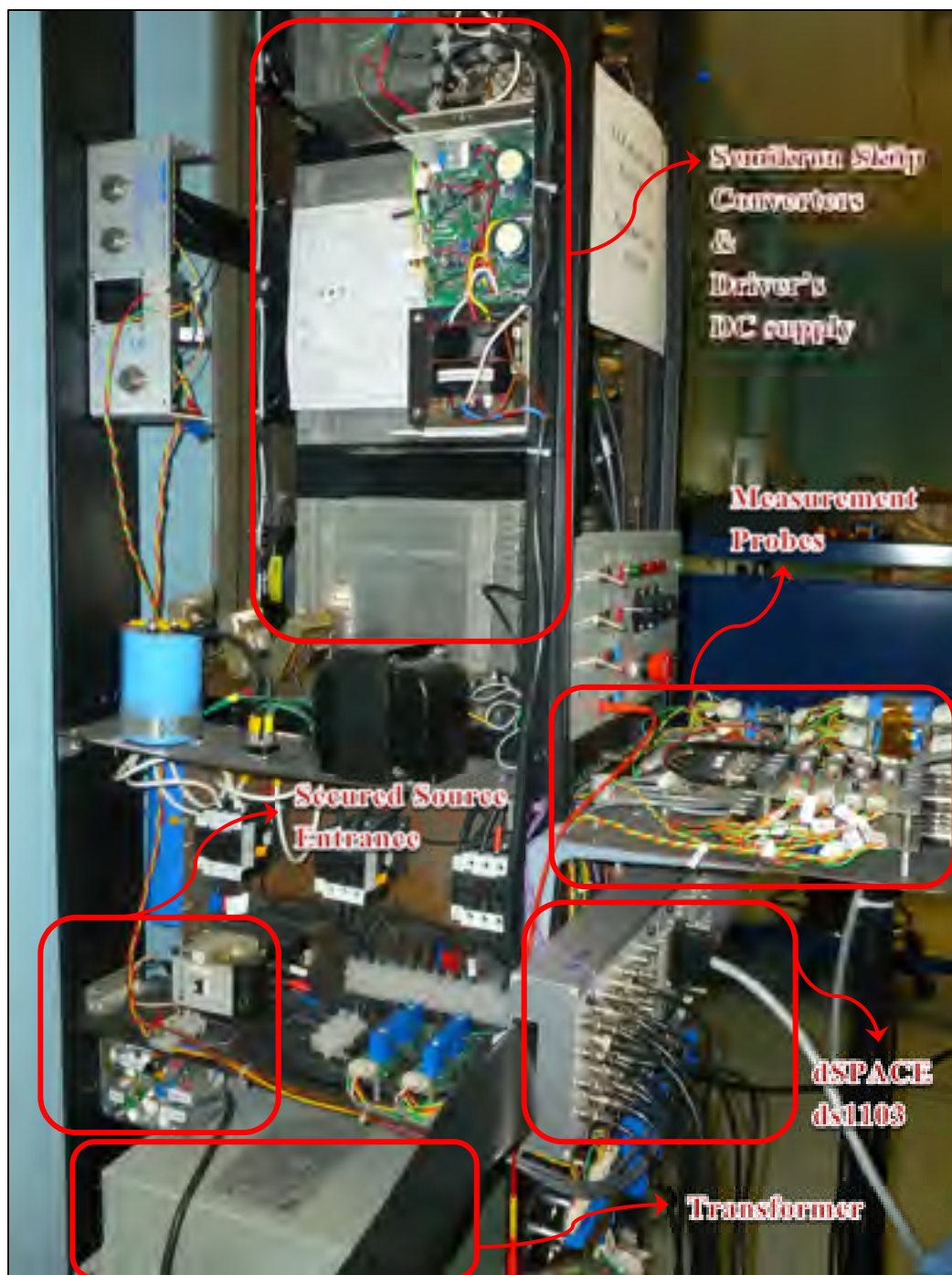
Figure 2.38 Experimental setup of 3P4W SeAF with isolating transformer
