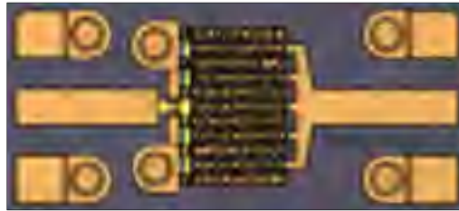
Figure 4.15 A W200N10 GaN HEMT on Si substrate
