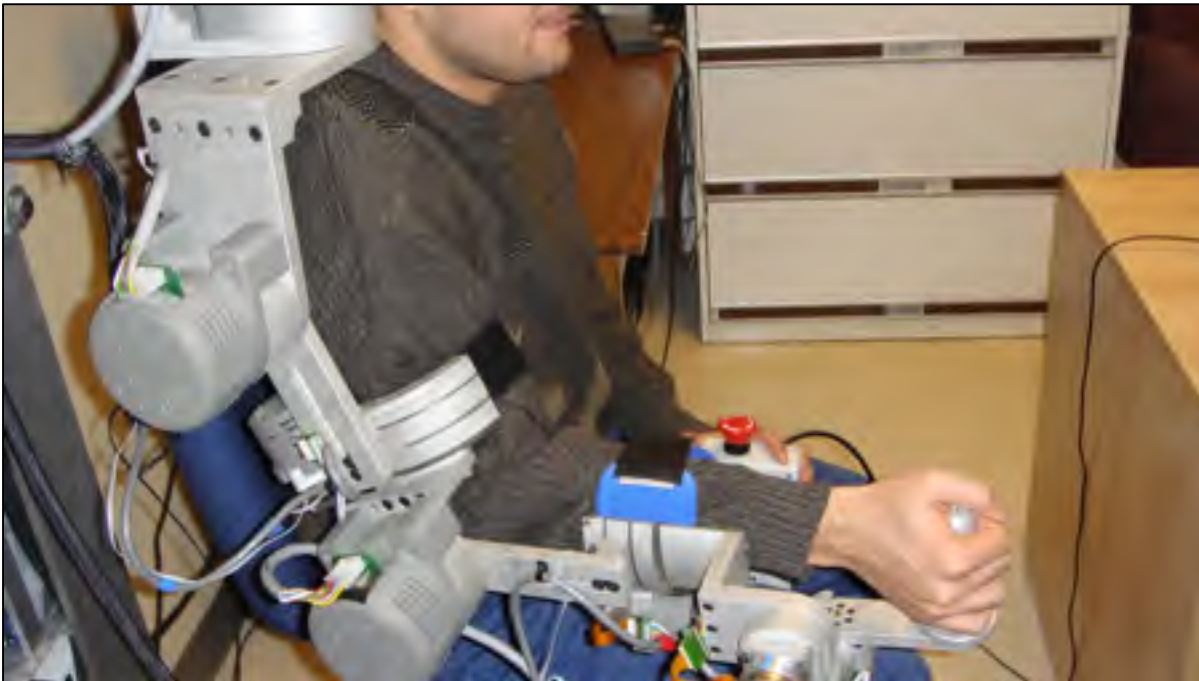
Figure 3.1 Subject wearing ETS-MARSE robot arm
