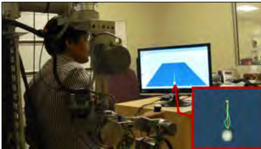
Figure 2.12 Experimental setup for active rehabilitation
