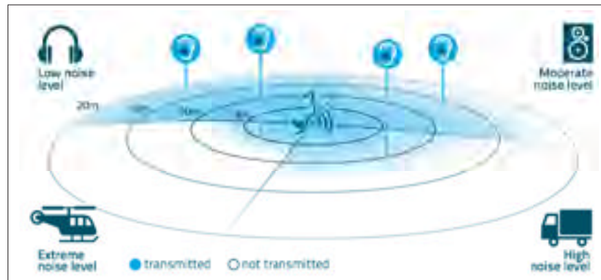
Figure 0.2 A graphic representation of the RAVE showing a talker and the potential distance of the transmitted signal based on the level of background noise.
