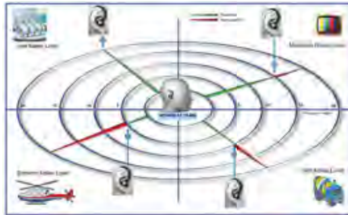
FIGURE 5: Illustration of functionality of RAVE. The green and red lines represent the areas where the signal is transmitted and not transmitted, respectively.
