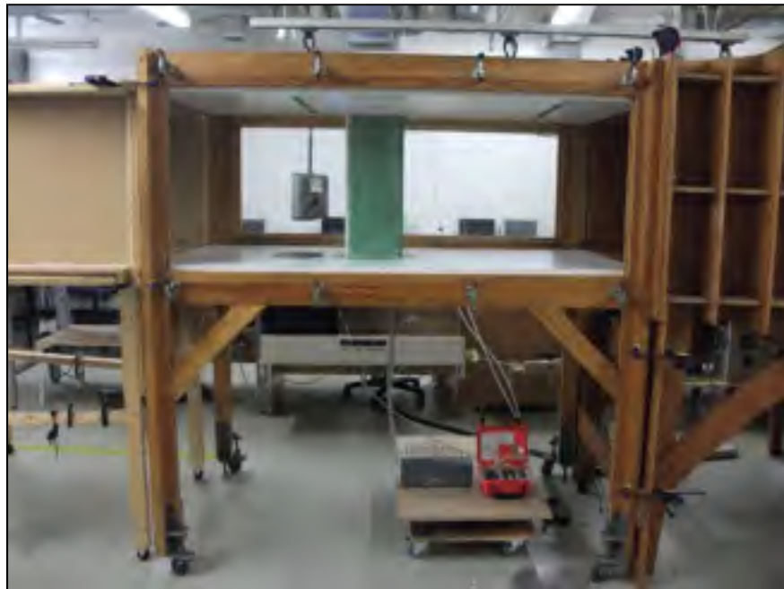
Figure 3.7 Original rigid model installed in the wind tunnel test chamber and connected to the AEROLAB measurement system
