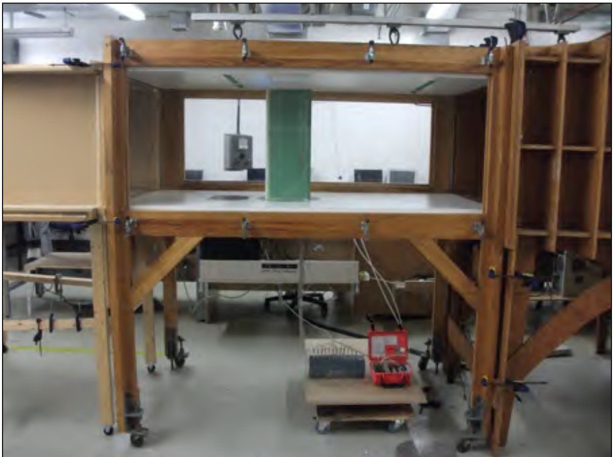
Figure 3.5 Wing model 4 installed in the wind tunnel chamber
