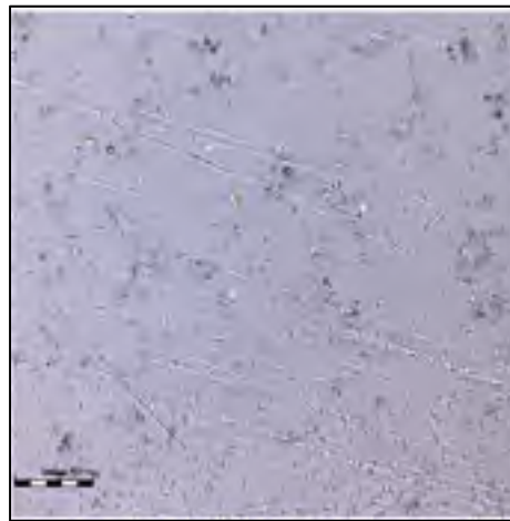
Figure-A I-2 Optical view of the dispersion in a 5 wt% CB epoxy composite; full scale bar = 100 \mu\text{m}
