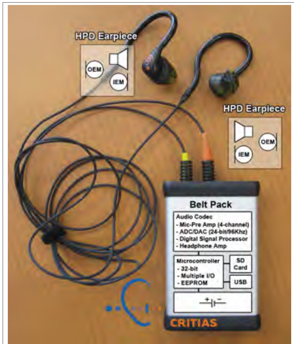
Figure-A V-1 First version of the Auditory Research Platform
