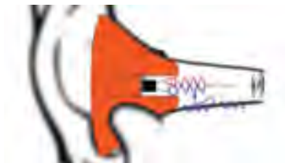
FIGURE 4: Active noise control of occlusion effect: noise in the ear canal is picked up by an internal microphone, and a cancellation signal is generated with the loudspeaker.
