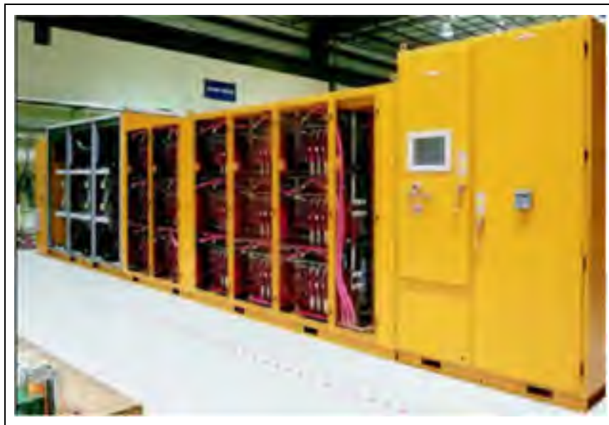
Figure 1.25 IGBT 11L-CHB drive by ASI Robicon
