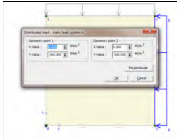
Figure 1.49 Assigning the load through the stage construction window
