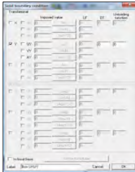
Figure 1.18 Solid boundary condition window, vertical fixities for bottom side
