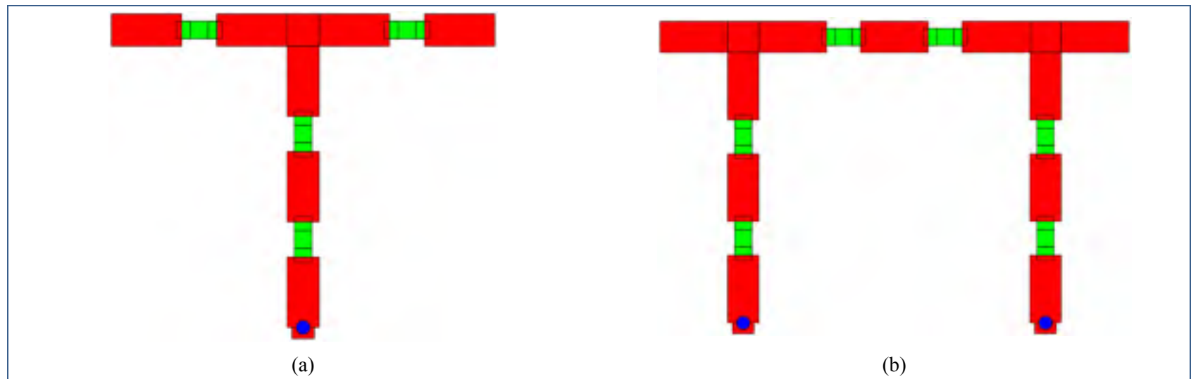
Figure 5.82 Resulting PM after granularity refinement: (a) T and (b) \Pi attenuator layouts
