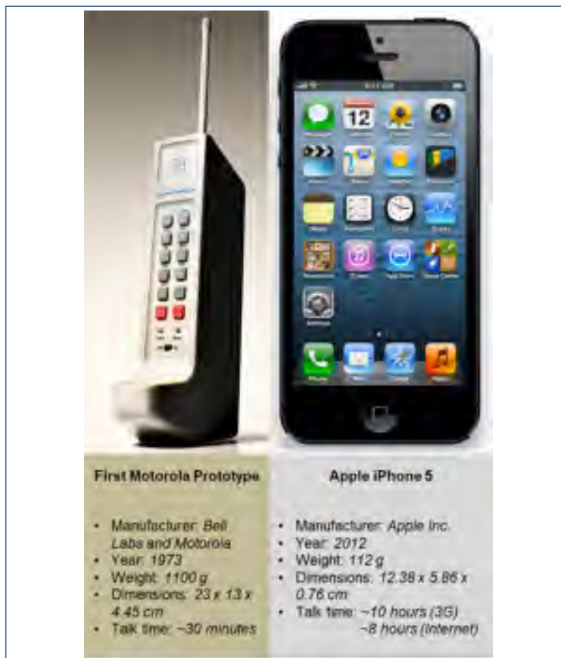
Figure 1.2 A comparison between the first handheld mobile phone and a recent smartphone
