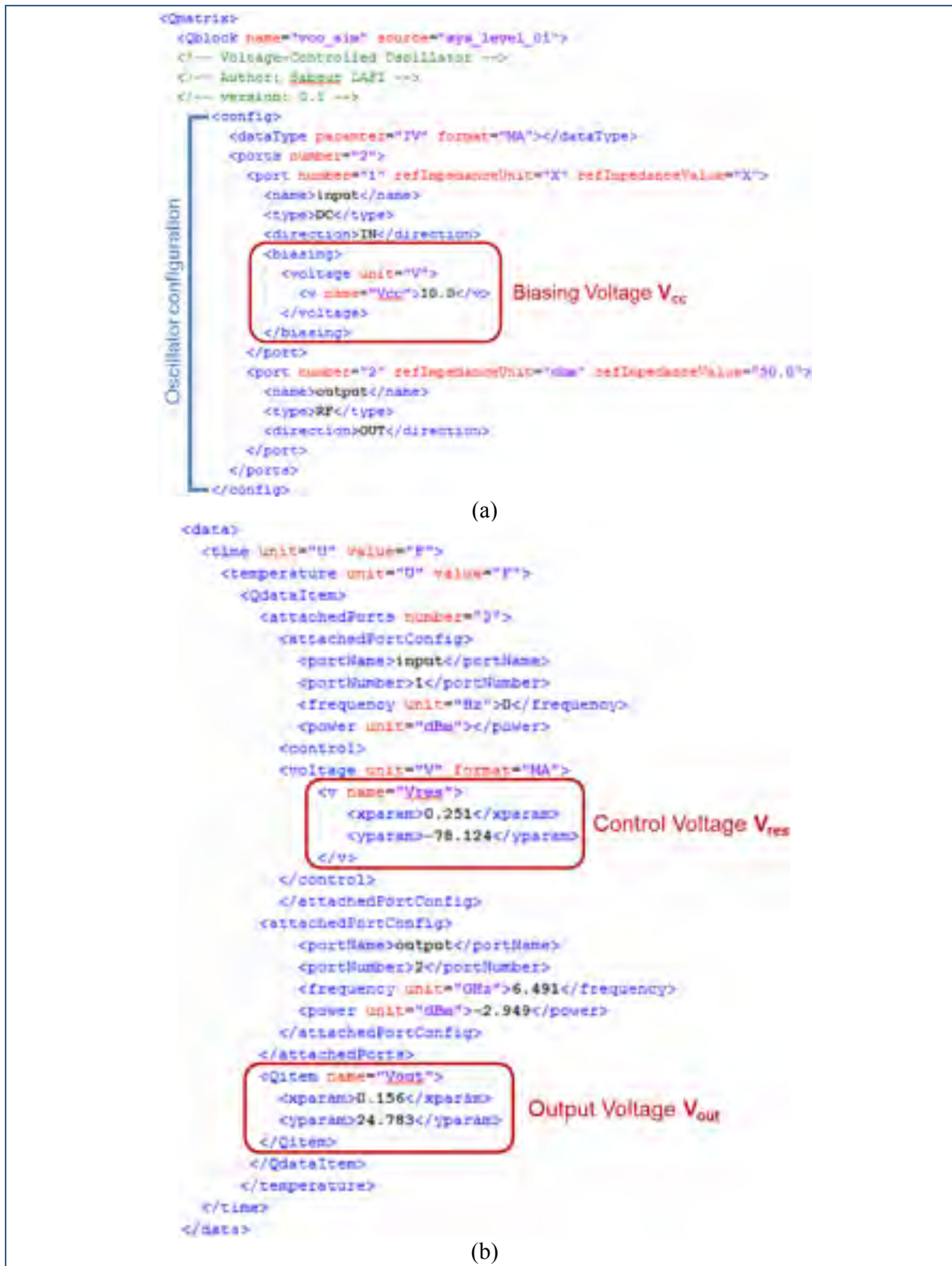
Figure 3.24 VCO's Q-matrix XML structure (cont'd): (a) the configuration section and (b) the data section (limited to only two points of control and output voltages)
