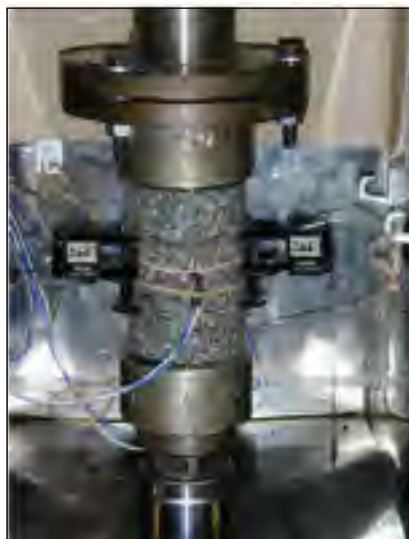
Figure 2.6 Uniaxial tension-compression complex modulus test setup
