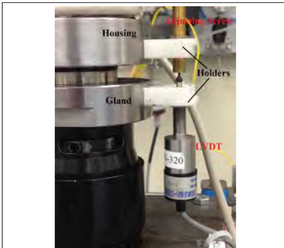
Figure 2.3 Displacement measuring mechanism
