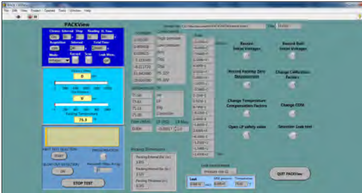
Figure 2.12 The LabView platform to control the packing test rig
