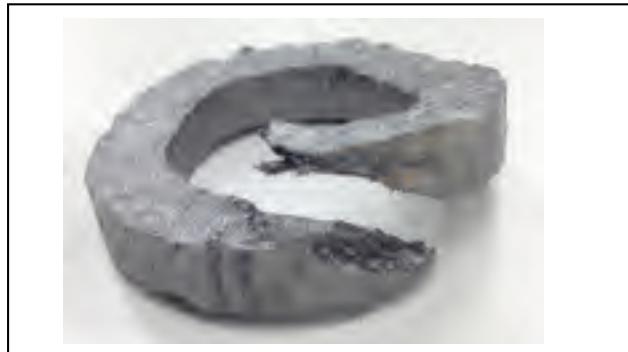
Figure 2.13 A flexible graphite plaited packing ring
