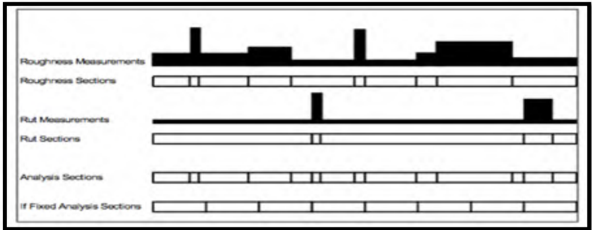
Figure 1.16 Dynamic Sectioning versus fixed sectioning approach Taken from Bennett and Paterson (2000)
