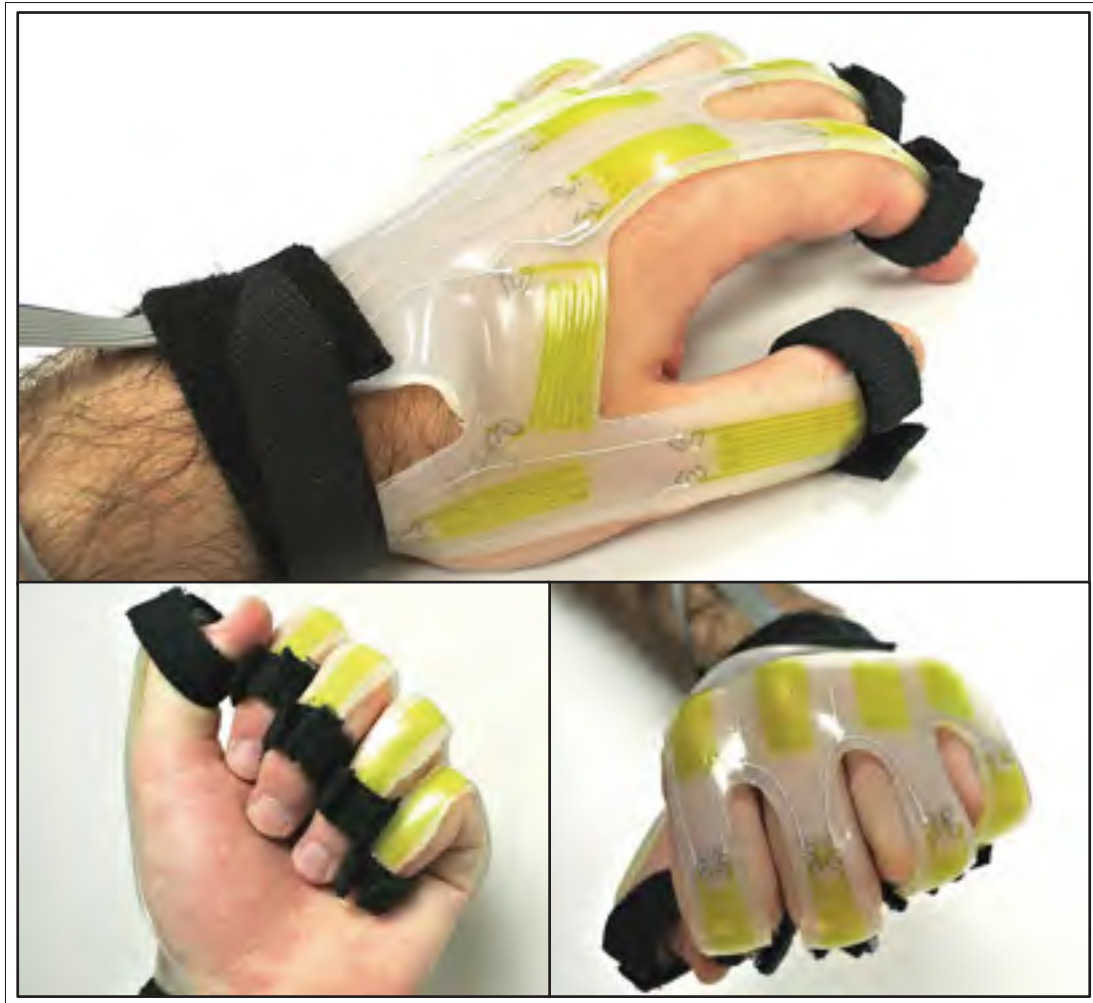
Figure 1.4 Wearable soft artificial sensing skin made of a hyperelastic elastomer material for detecting multi-joint motions.
