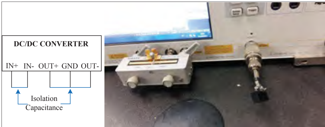
Figure 2.11 DC/DC converter isolation capacitance measurement
