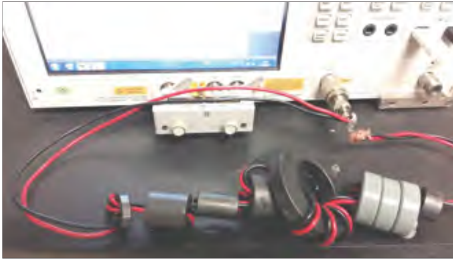
Figure 2.8 Ferrite cores to remove CM current
