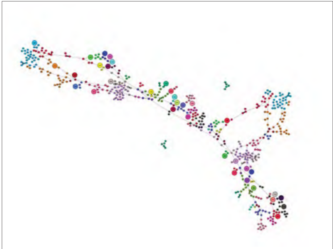
Figure 3.4 High Voltage transmission network for 5000 bus power grid. Larger circles represents selected pilot nodes. Different colors represent different areas
