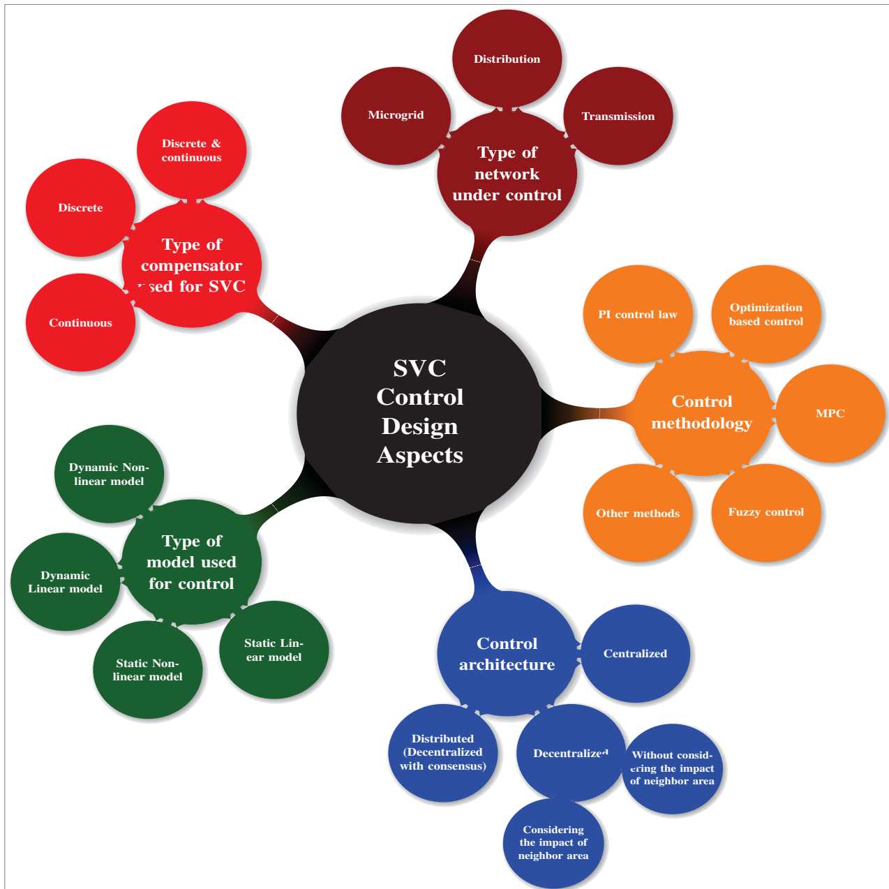
Figure 2.1 Classification of SVC Control desing aspects
