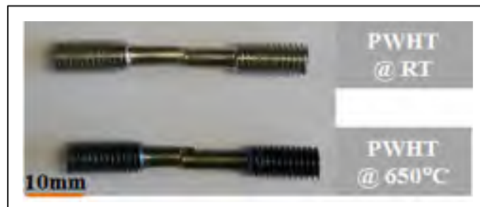
Figure 2.21 Fractured PWHT tensile samples of joint#4 at room temperature (RT) and 650 °C.
