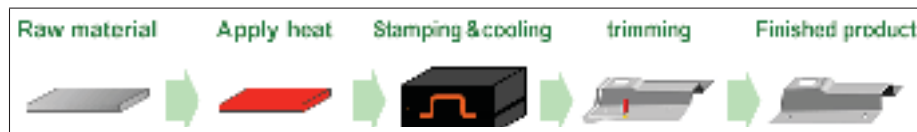
Figure 1.1 Main steps of the hot stamping process (Futaba Industrial, 2016)
