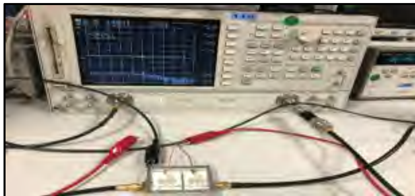
Figure 4.4 Real measurements setup of fabricated PA
