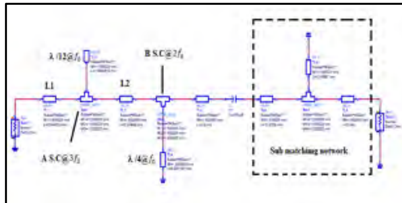
Figure 2.15 Output matching network
