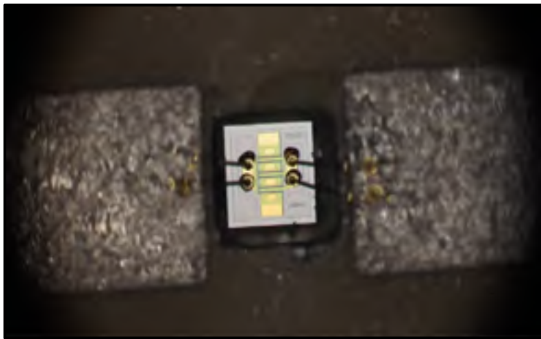
Figure 4.2 wire bound connection
