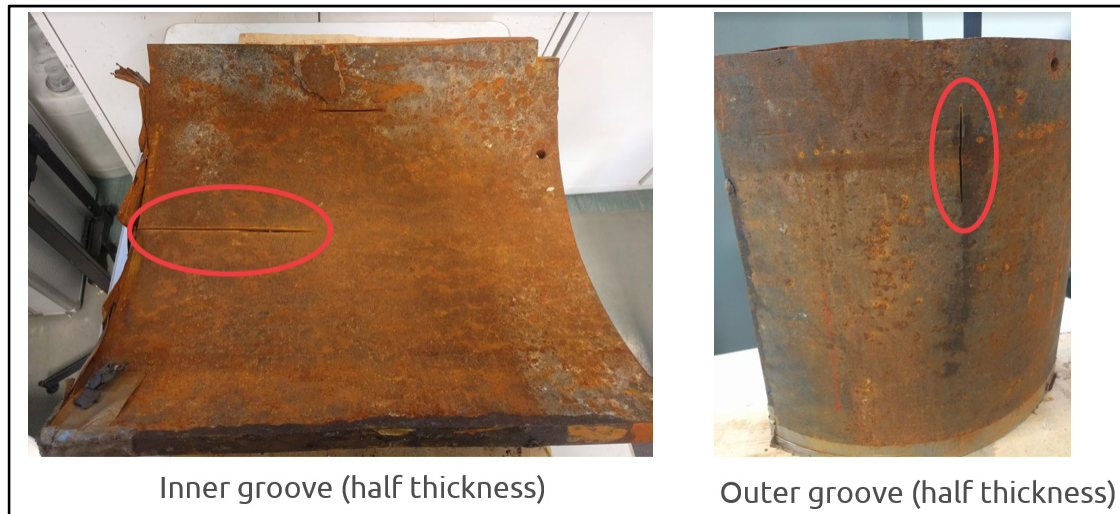
Figure 3.9 Machined grooves on inner and outer surfaces of the pipe sample
