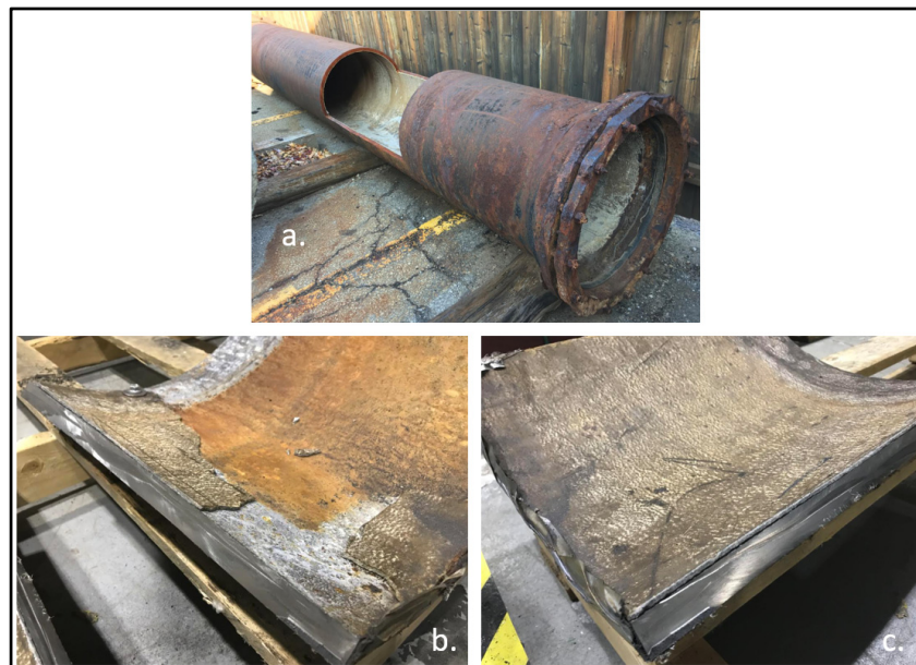
Figure 3.1 a. Pipe from which samples have been cut, b. Non-coated sample and c. Coated sample
