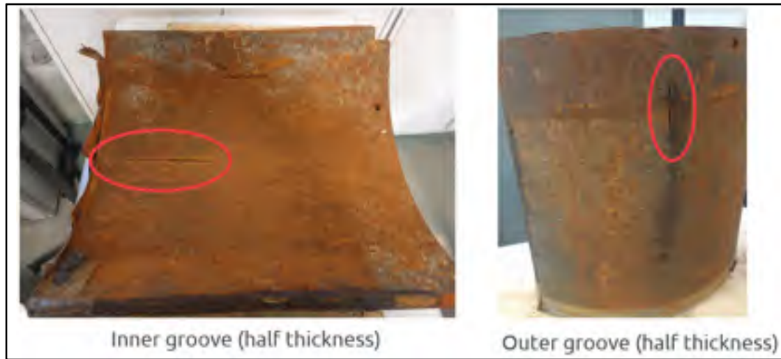
Figure 3.9 Machined grooves on inner and outer surfaces of the pipe sample
