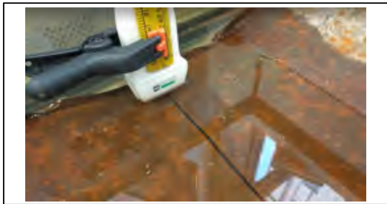
Figure 3.10 Array setup above the groove under inspection
