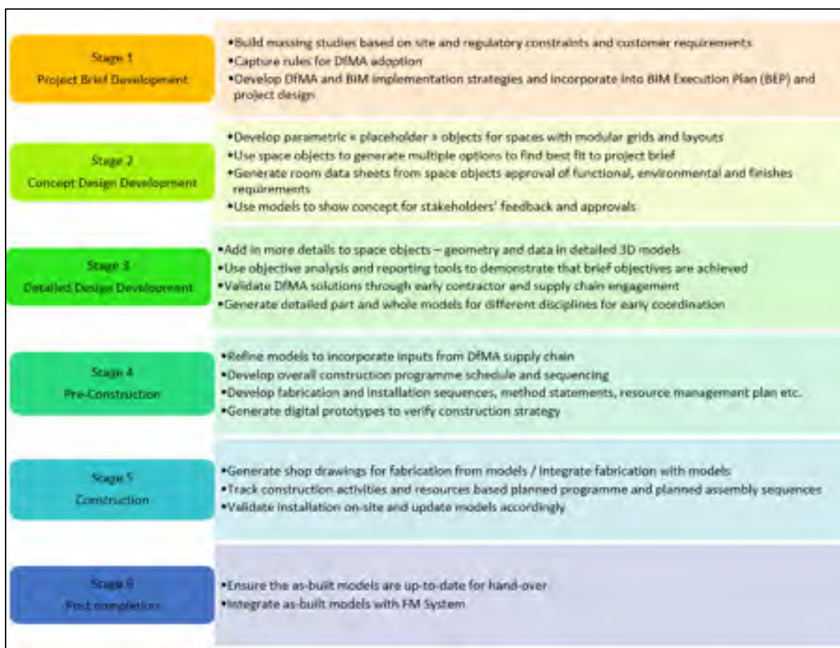
Figure 2.6 Key BIM actions for the DfMA approach at the various stages Adaptée de Bryden Wood – BCA (2016)
