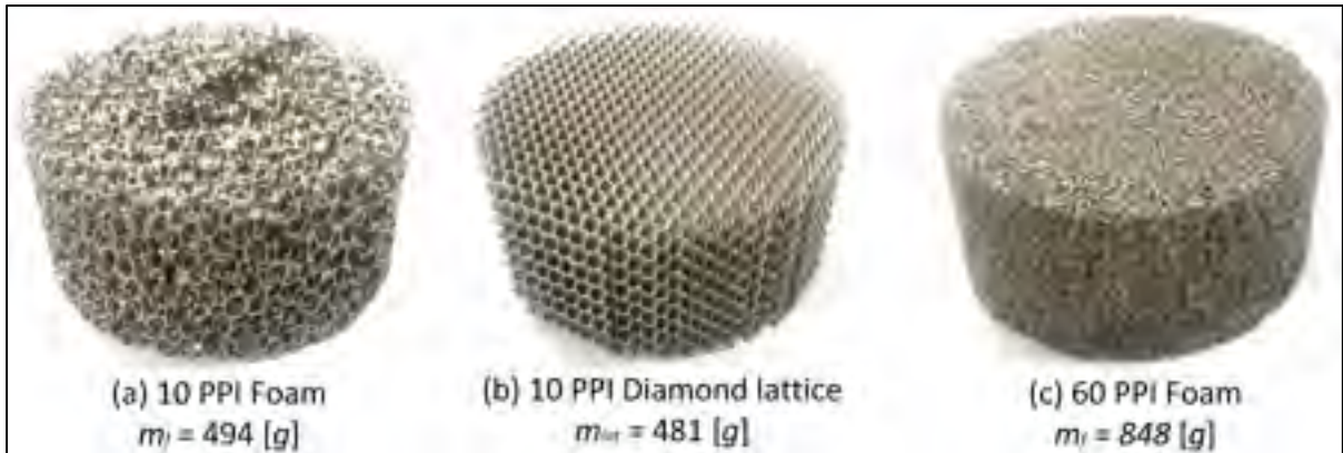
Figure 2.28 CoCr specimens after EDM cut
