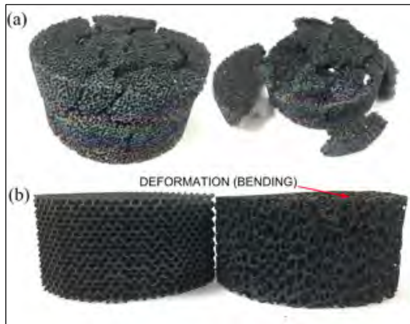
Figure 3.7 Failures after operation: (a) SiSiC : crack formation of the 60 PPI foam; (b) CoCr : Deformation, comparison between the 10 PPI lattice and foam structures
