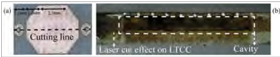
Figure 2.5 Photograph of fabricated E-LIW (a) completed structure (b) cut in the middle (at the cutting line) by laser in order to show the inner air cavity
