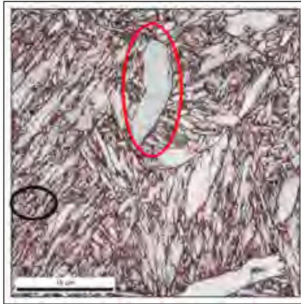
Figure 6.8 EBSD grain boundary map of HCr alloy steel deformed at deformation temperature of 1200 °C and strain rate of 1 s -1 . The HAGBs are shown in black and LAGBs are shown in red
