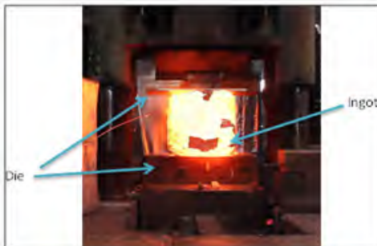
Figure 1.3 Forging Process in 5000-ton capacity press
