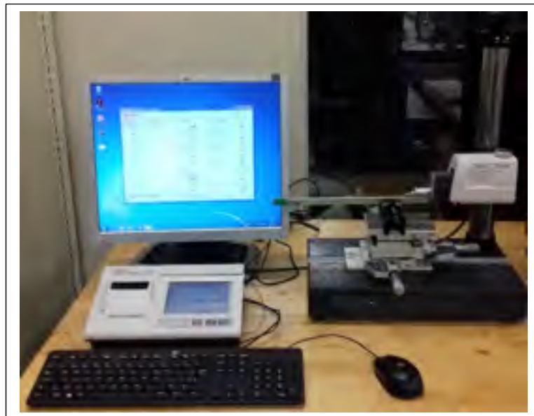
Figure 2.16 La machine Mitutoyo SJ400
