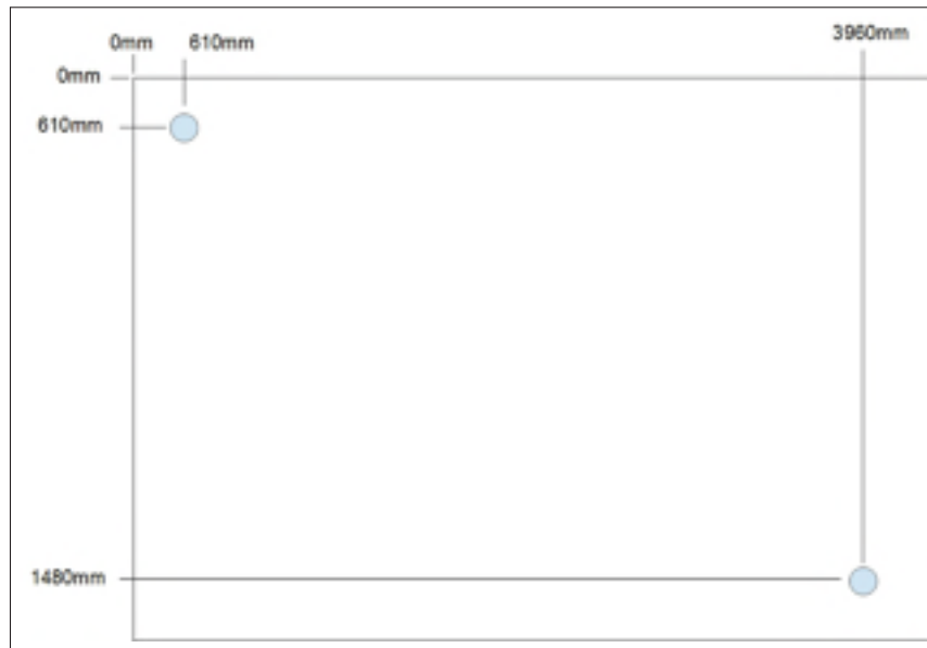
Figure 2.8 Thermocouples on walls with no heating system
