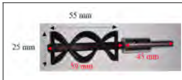
Figure 2.1 3D printed spindle into its shaft
