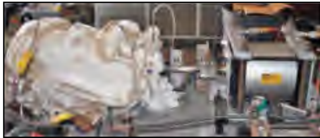
Figure 1.3 Test rig for API-622, (Davis, 2012)
