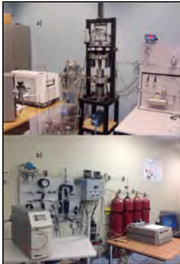
Figure 4.2 a) Gasket ROTT test rig and b) universal packing test rig
