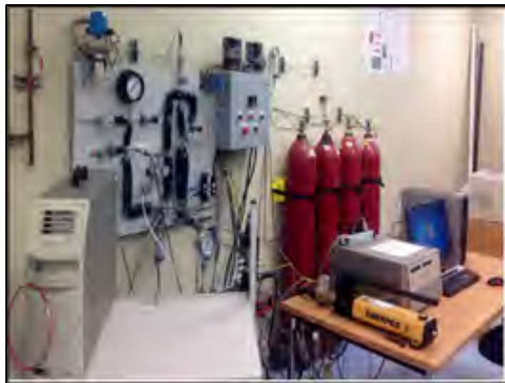
Figure 6.2 Universal packing test rig for gases
