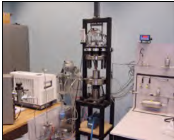
Figure 2.10 ROTT test rig
