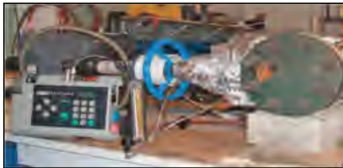
Figure 1.4 Test rig for API-624, (Davis, 2012)
