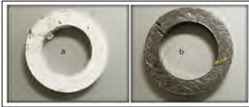
Figure 0.4 Packing ring a) PTFE b) Flexible graphite
