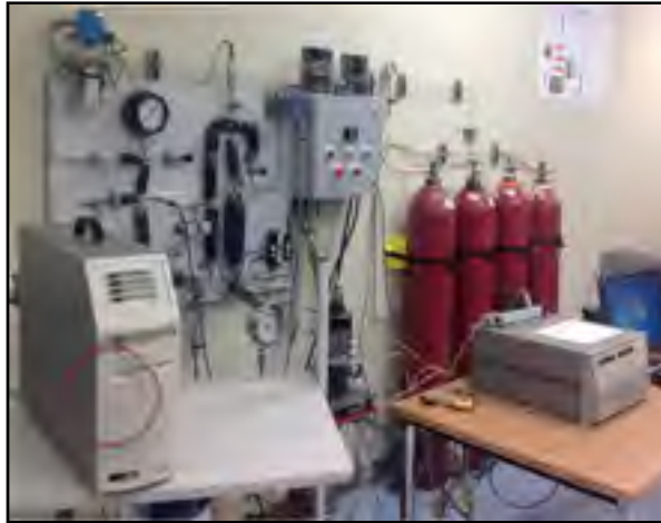
Figure 3.2 General configuration of the test bench for leak detection test
