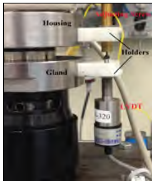
Figure 2.3 Displacement measuring system
