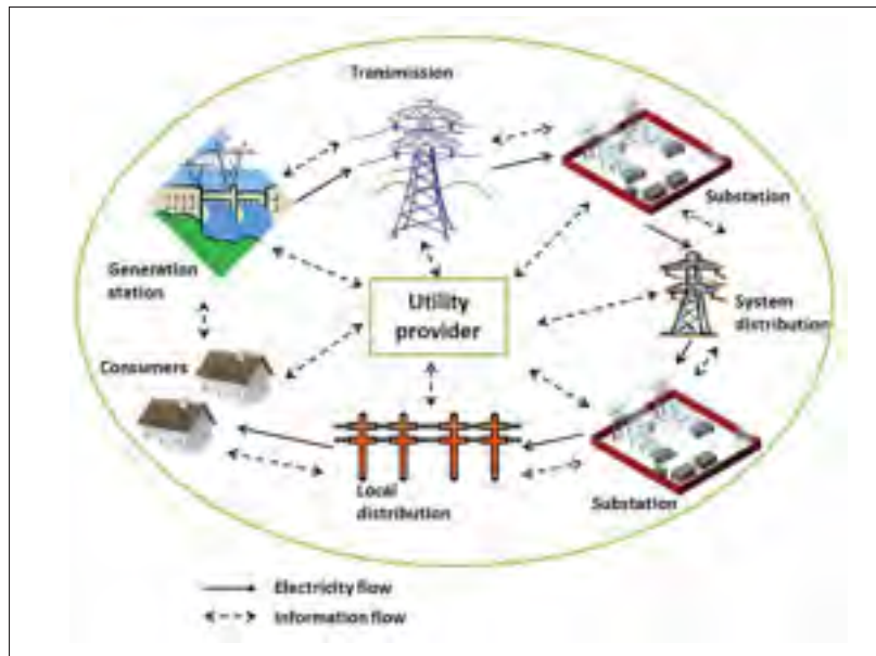
Figure 0.1 Illustration of the two-way electricity and information flows for smart grid scenario
