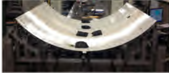
Figure 4.1 An aerospace panel restrained by known forces on its inspection fixture (Aidibe & Tahan, 2015)
