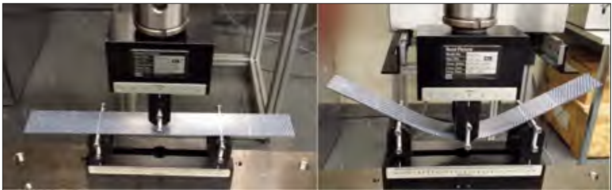
Figure 3.4 Three point bending test using the MTS machine
