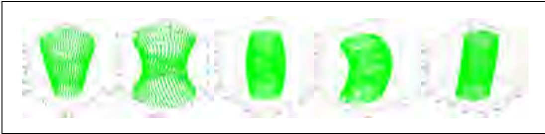
Figure 5. 9 Synthetic data with form error simulations on cylinder surfaces, n = 2000
