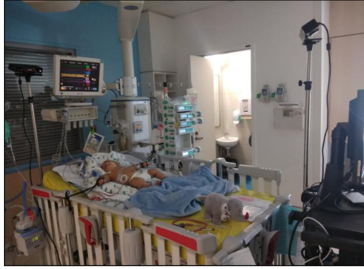
Figure 2-6 System setup and Kinect sensors locations during the experiment on a critically ill patient in the PICU of Sainte-Justine Hospital
