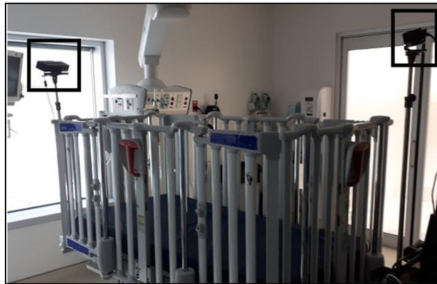
Figure 3-1 System setup: The locations of depth sensor are shown with the 2 frames
