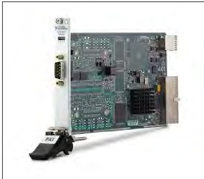
Figure F-1. NI PXI 8531 CAN open interface
