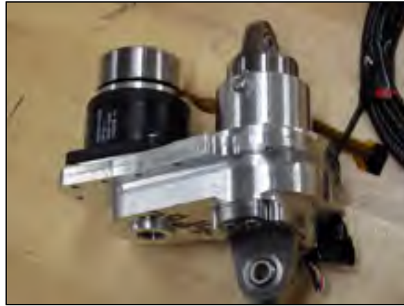
Figure 2.6 BLDC motor-based morphing actuator
