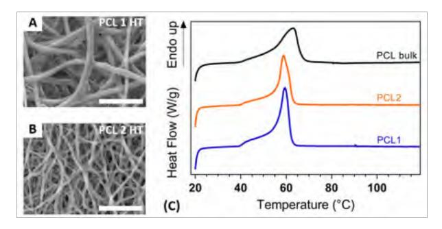
Figure 5.4 (A,B) SEM images of the morphology of PCL1 and PCL2 mats after heat treatment (scale bar: 30  $\mu$ m). (A) PCL1HT and (B) PCL2HT. (C) DSC thermograms of bulk and electrospun PCL.
