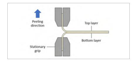
Figure 5.2 Representation of the T-peel test configuration
