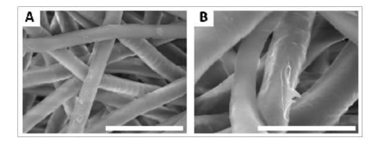
Figure 5.6 SEM images of PCL1 mats after a peel test showing defects on microfibers representing pieces of residual fibers from the other microfiber mat of the bilayer system. Scale bars: (A) 20 μm and (B) 10 μm.
