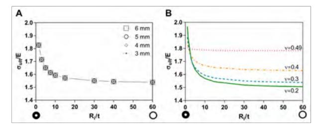
Figure 3.3 (A) Lower limit of the ratio of tensile ultimate strength to elastic modulus (σ<sub>ult</sub>/E) according to the ratio of the internal radius to wall thickness (Ri/t) to reach both compliance and burst pressure target values, respectively 0.0725 %/mmHg and 2031 mmHg. The Poisson's ratio was fixed as 0.3. Curves for VG with diameters of 3 to 6 mm are superposed.
