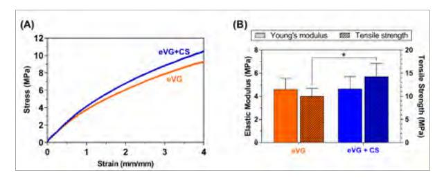
Figure 4.4 Mechanical properties of eVG and eVG-CS grafts. (A) Representative engineering stress-strain curves from circumferential tensile testing. (B) Mean elastic modulus and tensile strength (n = 13). Statistical difference noticed \* (p < 0.05).
