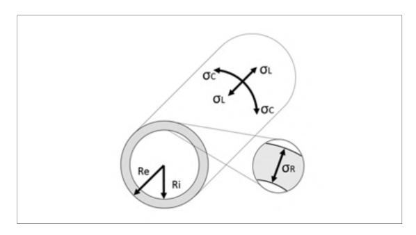
Figure 3.1 Schematic illustration of stresses involved in the model calculation.  $\sigma_C$ ,  $\sigma_R$  and  $\sigma_L$  represents respectively the circumferential stress, the radial stress and the longitudinal stress inside the cylinder with a fixed length and a uniformly applied internal pressure. The wall thickness t represents the difference between the external radius Re and the internal radius Ri.
