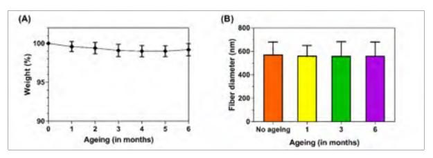
Figure-A 2B-1 Measurements of (A) weight and (B) fiber diameter of the eVG scaffolds as a function of ageing duration in a saline solution at 37°C over 6 months.
