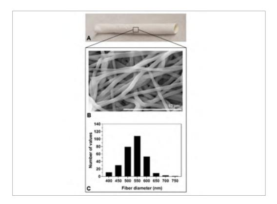
Figure 4.3 (A) Digital image of the graft. (B) SEM image of the nanofiber mat from eVG nanofiber mat (scale bar:  $10 \mu m$ ). (C) Distributions of fiber diameters for coated grafts. There was no difference between bare and coated materials.
