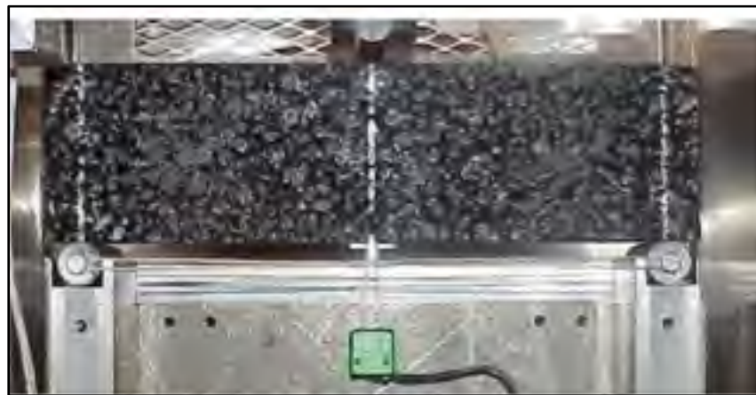
Figure 1.11 Essai de flexion 3 points (Wagoner et al., 2005)
