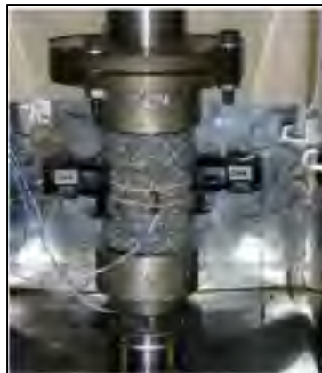
Figure 7.6 T- C complex modulus test setup.
