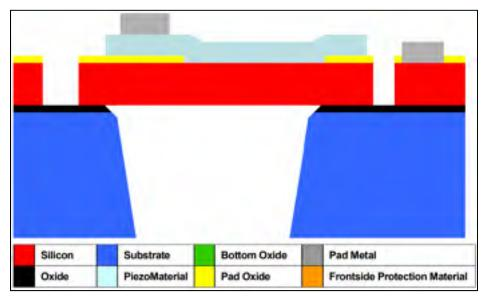
Figure 1.27 PiezoMUMPS crosss-section Taken from (MEMSCAP Inc., 2014).
