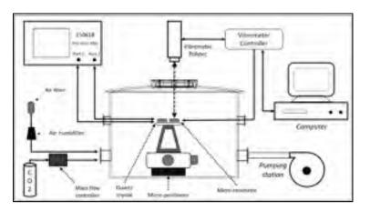
Figure 2.6 Diagram of the characterization setup
