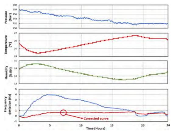
Figure 3.14 Long term test of the CO<sub>2</sub> MEMS sensor
