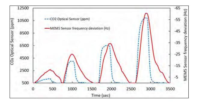
Figure 3.10 MEMS and optical sensor response to different CO<sub>2</sub> concentrations
