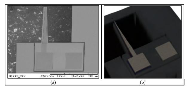
Figure 3.2 Uncoated micro-resonator (a) SEM micrograph, and (b) 3D view obtained by confocal microscope.
