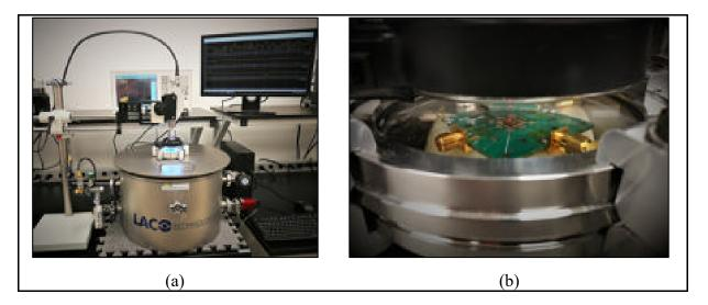
Figure 2.7 (a) Setup for the quartz crystals and the resonator characterization, (b) Close-up of the micro-resonator during the characerizacion with the laser from the vibrometer visible
