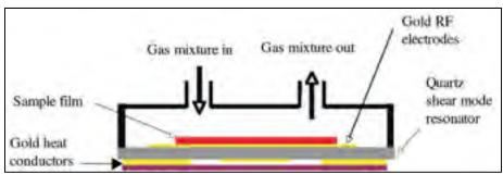
Figure 1.9 Piezoelectric sensors Taken from Smith (2007)
