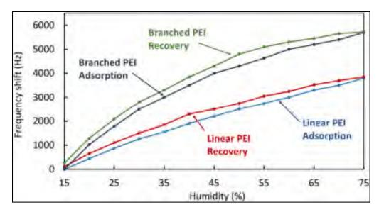
Figure 2.11 Branched PEI and Linear PEI coated crystals
