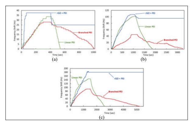
Figure 2.13 Response of the three different coatings at CO<sub>2</sub> concentrations of (a) 0.1%, (b) 0.5%, and (c) 1%
