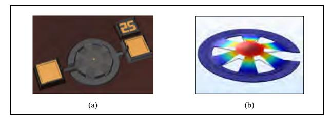
Figure 2.9 (a) 3D view of the real micro-resonator obtained by the Olympus LEXT OLS4000 Confocal microscope, (b) Eigenfrequency FEM COMSOL simulation
