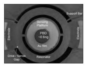
Figure 1.20 Disc micro-resonator Adapted from Konno et al. (2011)
