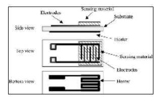
Figure 1.4 Polymer sensor diagram Taken from D. D. Lee (2001)
