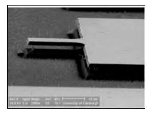
Figure 1.22 Electrostatic cantilever Adapted from Han et al. (2018)
