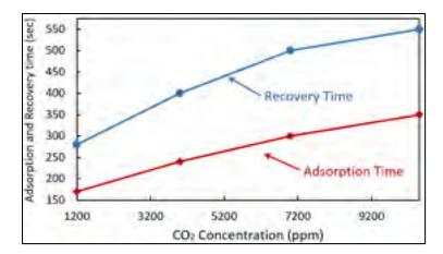
Figure 3.11 Adsorption and Recovery times based in the CO<sub>2</sub> concentration
