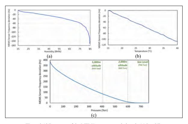
Figure 3.13 Response of the MEMS sensor to variations in (a) humidity, (b) temperature and (c) atmospheric pressure.
