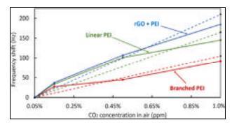
Figure 2.14 Frequency shift of each coating from 0.05% to 1% of CO<sub>2</sub>
