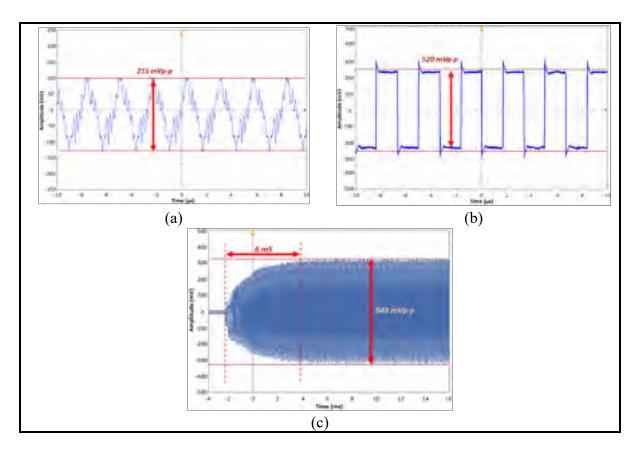
Figure 3.8 Measured CO<sub>2</sub> MEMS sensor signal waveforms at the different points labelled in Fig. 3.7 steady-state at (a) P1 and (b) P2, and (c) startup transient of the resonator at P3.
