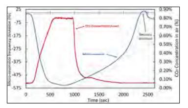
Figure 2.17 Response of the coated micro-resonator to a 0.8% CO<sub>2</sub> concentration variation
