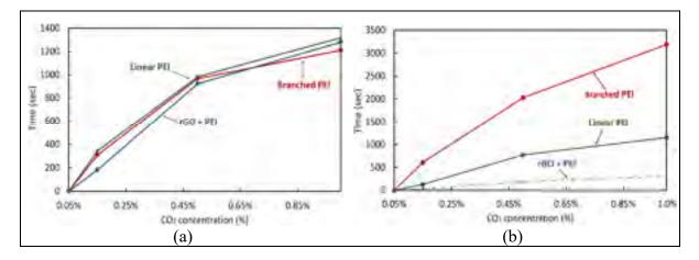
Figure 2.15 (a) Adsorption time for each coating at different CO<sub>2</sub> concentrations, (b) Recovery time for each coating at different CO<sub>2</sub> level
