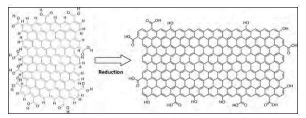
Figure 2.3 Reduced Graphene Oxide by Microwave reduction
