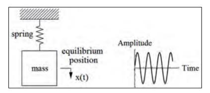
Figure 1.10 Undamped system diagram Adapted from Layton (2010)
