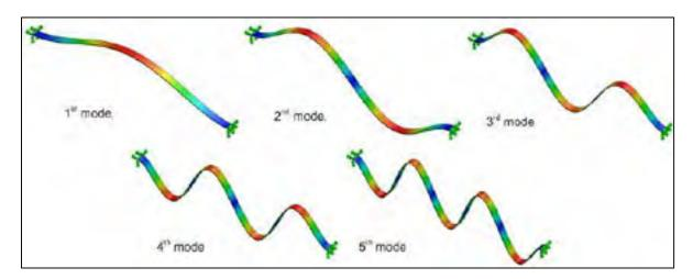
Figure 1.16 Resonant modes of MEMS bridge Adapted from Zaman et al. (2014)
