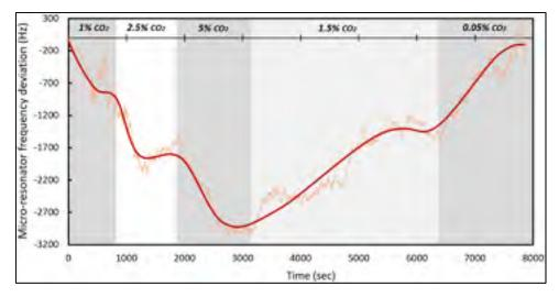
Figure 2.18 Behavior of the micro-resonator over time at different concentrations of CO<sub>2</sub>
