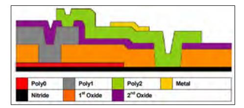
Figure 1.25 PolyMUMPS lateral cut representation Taken from (MEMSCAP, 2011).
