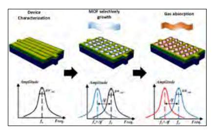
Figure 1.15 Frequency deviation diagram Adapted from MIT (2016)
