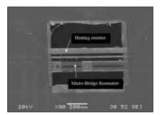
Figure 1.23 Electro-thermal micro-resonator Adapted from (Han et al., 2018)
