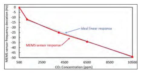
Figure 3.12 MEMS sensor frequency deviation by CO<sub>2</sub> concentration
