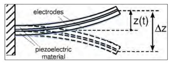
Figure 1.26 Piezoelectric MEMS resonator operation Taken from Romani, Sangiorgi, Tartagni, et Paganelli (2011)
