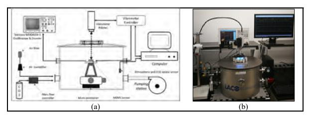
Figure 3.6 (a) Diagram of the characterization setup, (b) Setup for the CO2 gas sensor characterization
