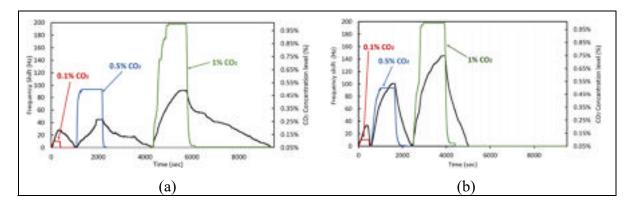
Figure 2.10 Quartz crystal frequency shift in response to different CO<sub>2</sub> concentration cycles for (a) Branched PEI coated crystal, and (b) Linear PEI coated crystal
