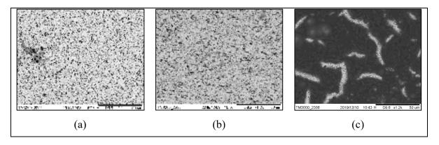
Figure 2.4 SEM image of the quartz crystal coated with the (a) Branched PEI layer, (b) Linear PEI layer and (c) rGO with Linear PEI layer
