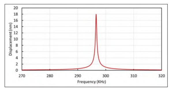
Figure 3.5 Vibrometer measurement after the LPEI coating deposited
