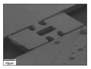
Figure 1.19 Free-Free beam micro-resonator Adapted from Hajjam et Pourkamali (2012)
