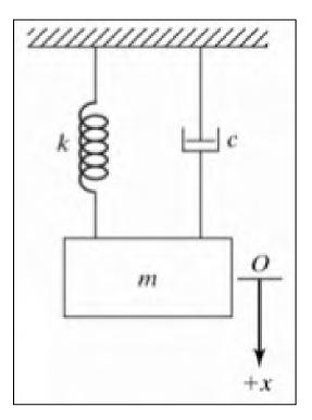
Figure 1.11 Damped system diagram Adapted from Layton (2010)
