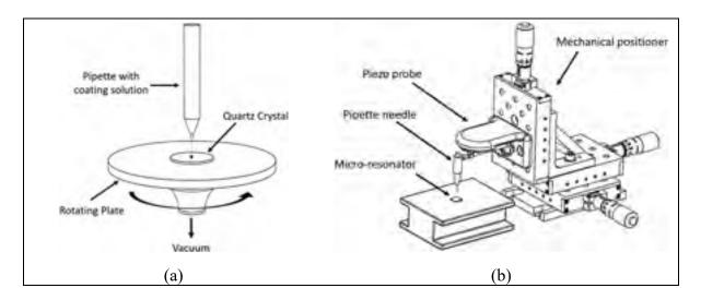
Figure 2.2 Coating deposition technique, (a) Spin coater for the Quartz Crystal used for initial coating tests, (b) Micro-drop deposition by piezo probe used for the micro-resonator
