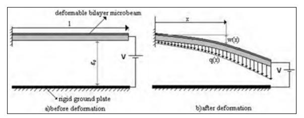
Figure 1.24 Electrostatic MEMS resonator operation Taken from Pashapur, Pesteii, Rezazadeh, et kouravand (2009)
