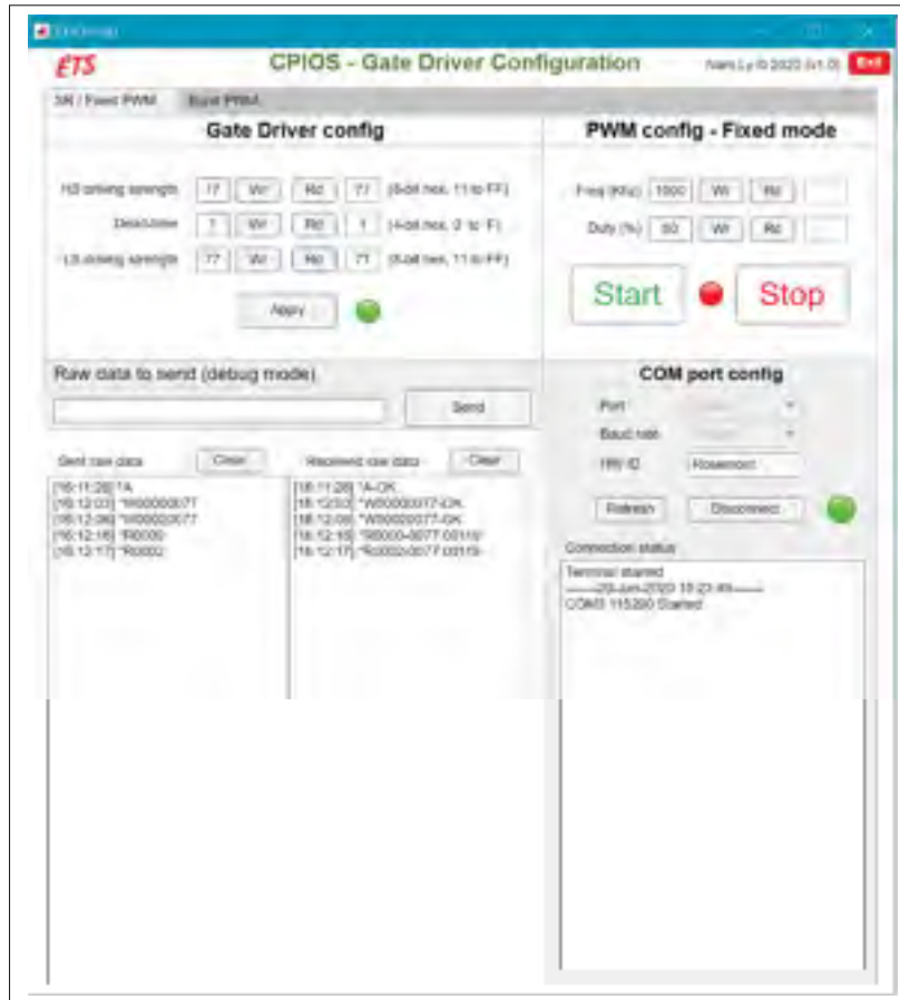
Figure 4.2 Matlab GUI of gate driver configuration and fixed PWM mode
