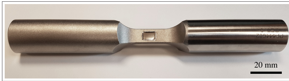
Figure 4.2 Final surface of the 8 A specimen's electropolished pocket
