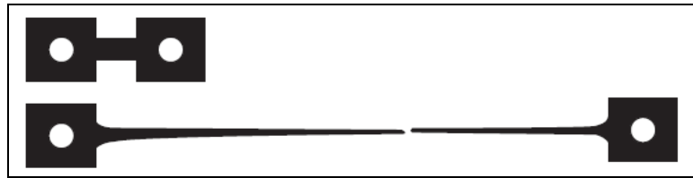
Figure 1-1 Super plastic titanium alloy before and after deformation (Gillo Giuliano, 2011)
