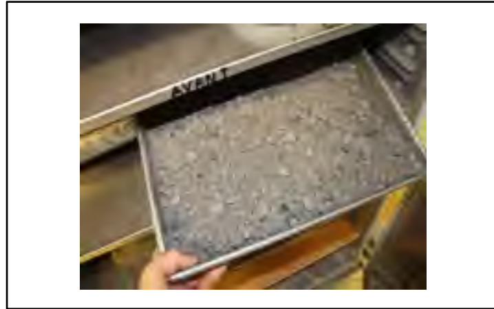
Figure 3.4 RAP drying in the chamber
