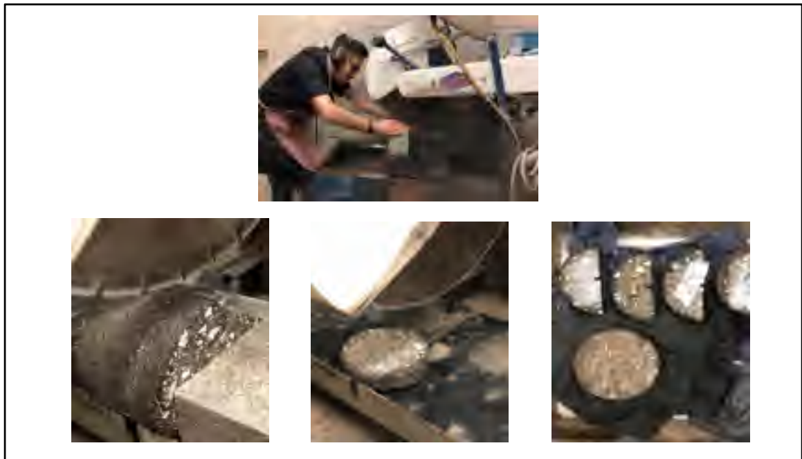
Figure 4.4 Specimen trimming for SCB test
