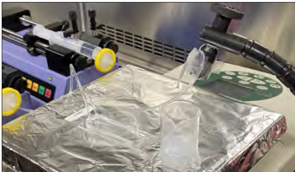
Figure 2.5 Microfluidic device connected to the syringe pumps
