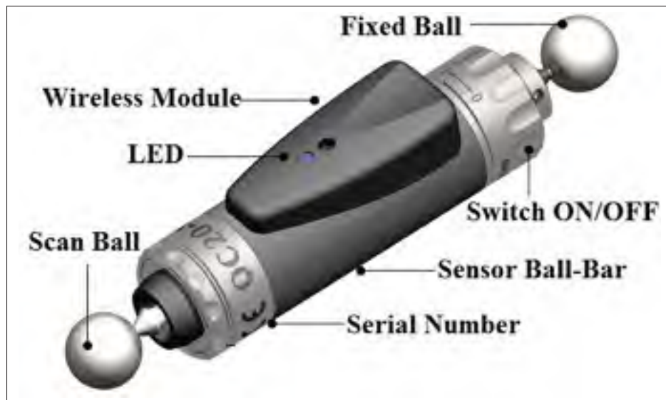
Figure 3.4 The QC20-W ballbar sensor Taken from Čep et al. (2018b)
