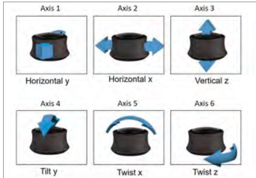
Figure 3.21 The SpaceMouse reference coordinate frame Taken from 3dconnexion (2020)
