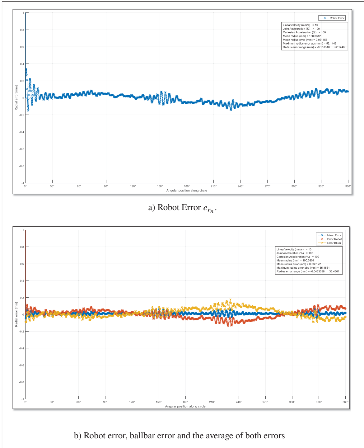
Figure 3.16 Error graphs when e_{equ_n} is equal to the average of both robot and ballbar error values
