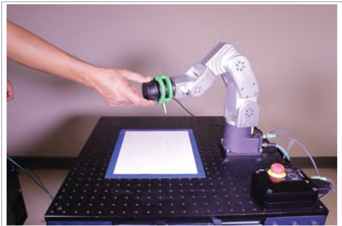
Figure 3.22 Experimental setup featuring the Meca500 six-axis industrial robot and the SpaceMouse Module from 3Dconnexion company
